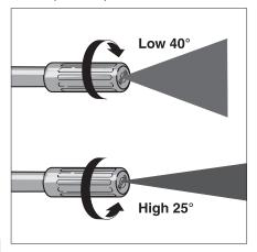
Turn the wand nozzle clockwise for high pressure. Turn counter clockwise for low pressure.
